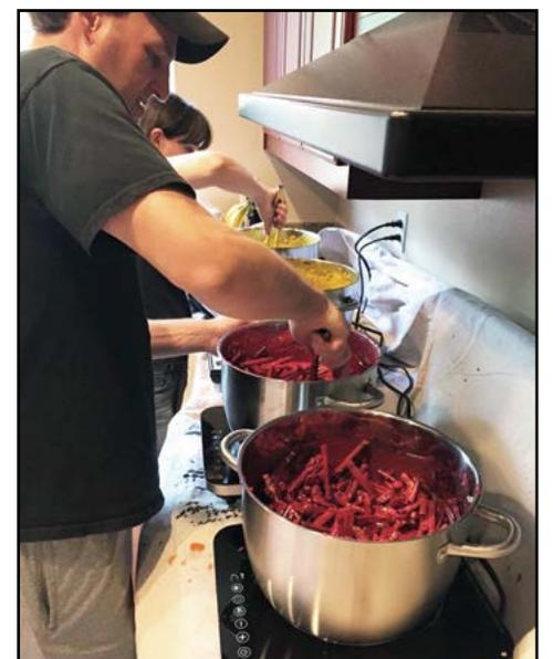
*Sorted by color, crayons are melted over induction burners. Testing has proven the process kills germs. Photo courtesy of TCI.*
